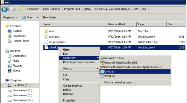
2. Search for the line that specifies the purge schedule in a standard cron format and edit the time value in a 24-hour format. For example, if you want to set your grooming for 8:00 PM of the 14th day of the month, the cron should be set at: **0 20 14** \* \* in a standard cron format. Check the images below.
