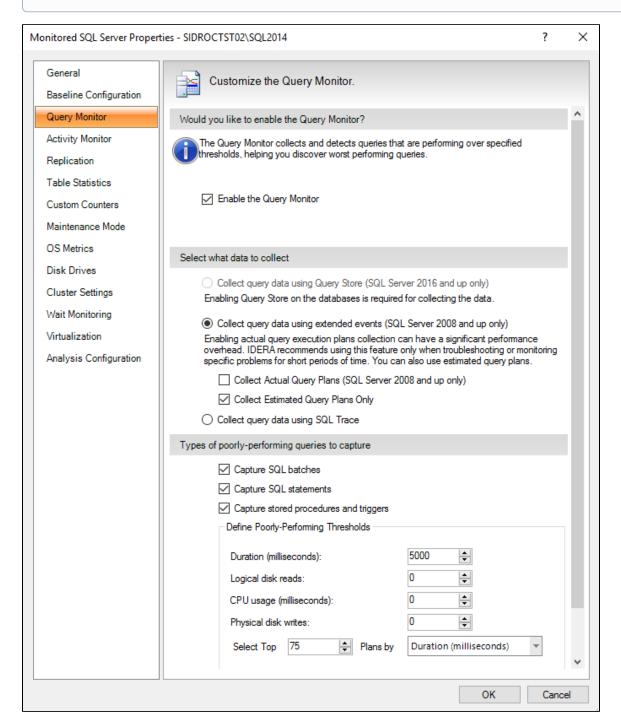
The Query Monitor window allows you to enable or disable query monitoring using the **Enable the Query Monitor** check box. You can also select the settings that are used:
