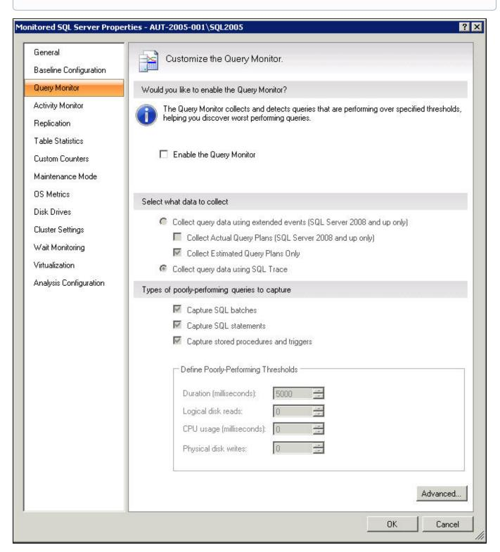
The Query Monitor window allows you to enable or disable query monitoring using the **Enable the Query Monitor** check box. You can also select the settings that are used:
