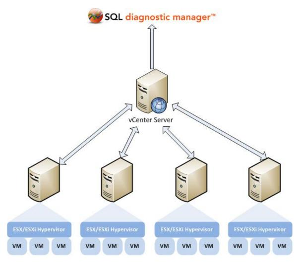
In virtualized environment with Hyper-V, the process of how SQL Diagnostic Manager collects and presents metrics is slightly different from that of a VMware setup. In this environment, SQL Diagnostic Manager collects all the required performance statistics from the Hyper-V host server and virtual machines using the WMI interface. See Hyper-V user requirements for information on how to successfully collect host and VM metrics.
