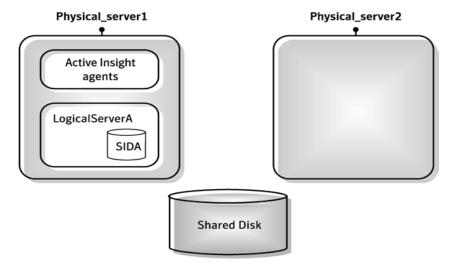
The following figure illustrates the live standby configuration after a failover.
