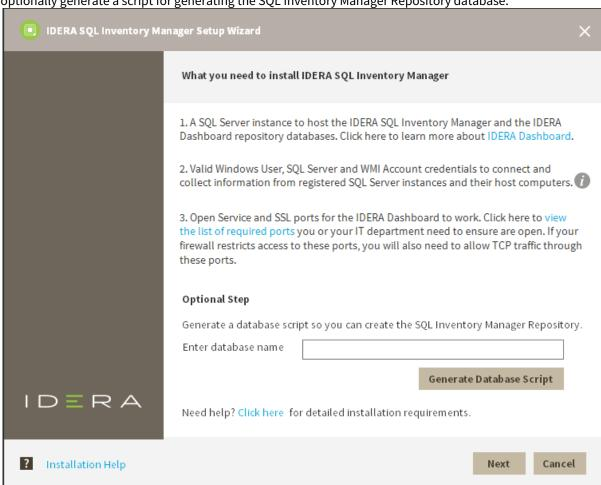
2. You must verify that the Firewall allows TCP (Transmission Control Protocol) traffic through **The ports you want to use**. By default, IDERA SQL Inventory Manager uses ports 9275 and 9291 for the Collection and Web Application services respectively.
