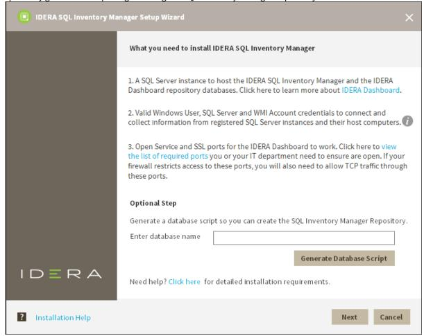
2. You must verify that the Firewall allows TCP (Transmission Control Protocol) traffic through **The ports you** want to use. By default, IDERA SQL Inventory Manager uses ports 9275 and 9291 for the Collection and Web Application services respectively.
