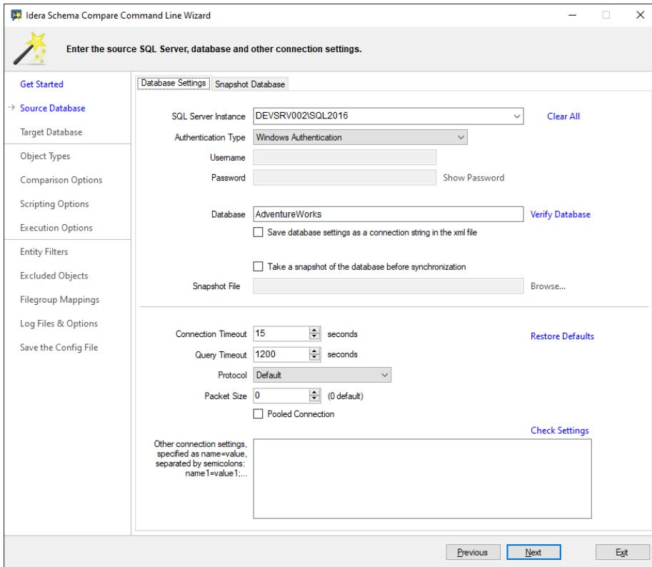
**i** Even though we refer to the SQL Server database as the "source" or "target", the command line can switch them, so the source can become the target and vice versa. More details on setting the target database are included in the Log Files and Options step.
