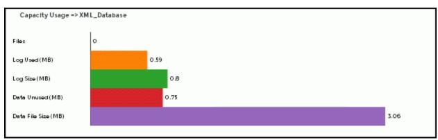
You can choose to view how data or the log is used on your database (in megabytes). Click any database in the top panel and the Capacity usage chart displays. This chart provides information on the number of files, Log Used (MB), Log Size (MB), Data Unused (MB), and Data File Size (MB).
